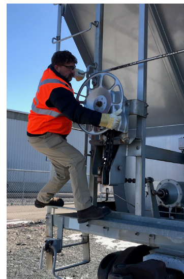
3-point contact for applying a vertical handbrake
