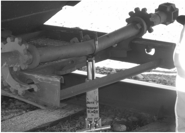
Bent hopper gate being repaired
